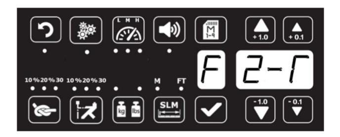
This function resets the calibration of machine to original factory calibration.
