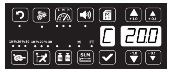
Pull a string. Check the value on tension meter. Adjust tension displayed on machine with Up /Down
