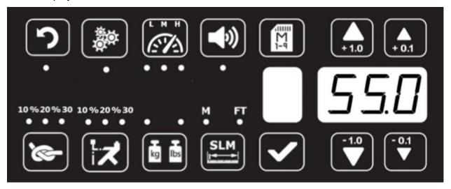
Touch the Knot button to tie off with 10, 20 or 30% extra tension. (To activate, touch the button short, to change % hold button longer (approx. ½ second), default is 10%). After touch the knot button, the display shows the 10% extra tension to be pulled:
