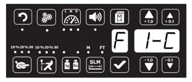
Touch enter button to start Calibration, then the screen shows as below to start Calibration.
