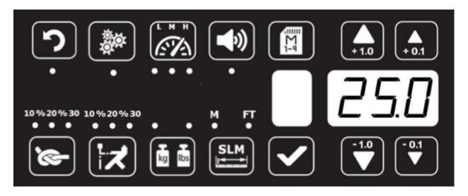
LB – KG setting is a "global" setting and can be changed at any moment. (Even during Calibration).
