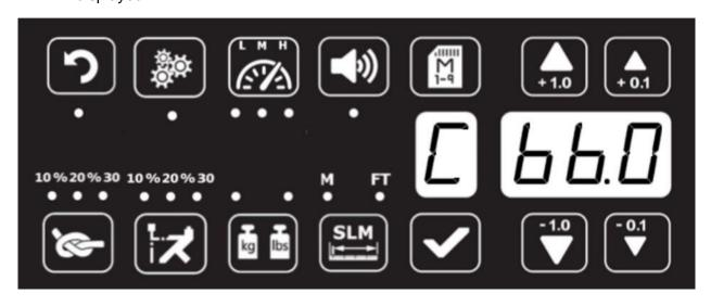
Pull a string. Check the value on tension meter. Adjust tension displayed on machine with Up /Down
