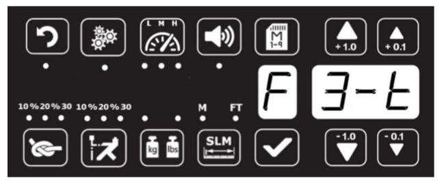
This function can modify the sensitivity of the activation metal touch switch. WARNING: Do not adjust if metal activation switch works fine.
