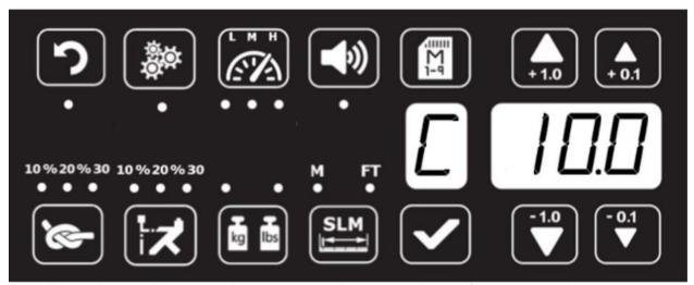
To calibrate the machine a tension meter must be mounted, start from screen above.
