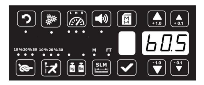
The LED light above knot button lights up, until the string is tensioned. This function works for one single time only.
